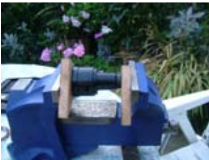
Pressing in new seal
